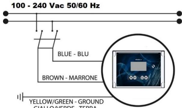
Fig. 1 – Electrical connection
