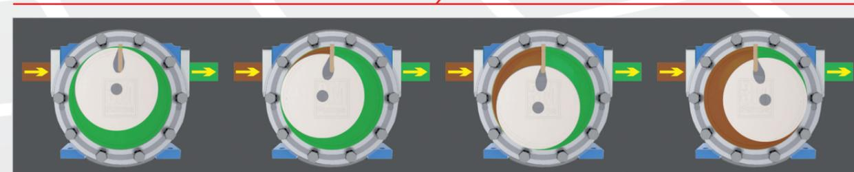
The hollow disc is eccentrically mounted in the rotor shaft and turns around the suction and discharge camera separator vane. In this way the piston is obliged to follow the trajectory around the vane and externally to the pump head, where it is pushed via an elastic device internally inserted.
